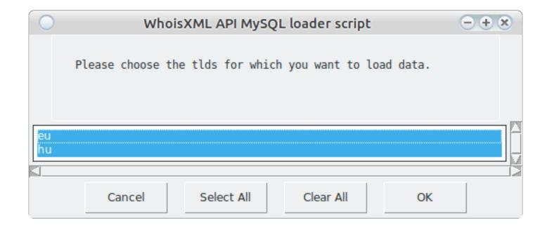
Finally, we get a text window showing what will happen next. If we press "OK", all windows will disappear and we can follow the progress in the terminal or console. This can take time. For large domains such as com, the time maybe even unacceptable. So having understood the concepts with the GUI approach, we may go for the BASH scripts which are more efficient, but less portable, unfortunately.
