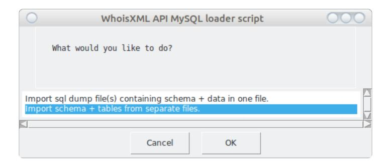
When we choose the first option, the script will use the files in which all data for a tld are saved into the same file. In the case of the second, each table will be loaded from a separate file. (The files for both approaches are downloaded by the downloader script.) Let we choose the second option as it is more efficient also for slightly bigger databases (and really big ones, too, if you use the BASH version of the script).
